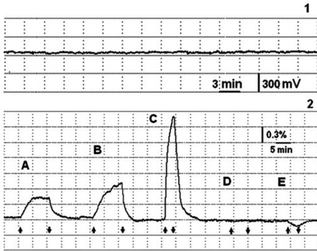
**FIG. 3.** BIOSCOPE's signals from different objects when there is a noncoherent light source. **A**, apple; **B**, grapefruit; **C**, human palm; **D**, aluminum plate at ambient temperature; **E**, same plate heated to 40°. Distance between all objects and BIOSCOPE is 1 cm. Arrows show the moments of placing and removal of objects on/from the sensor. Numbers at the square indicate the scale.
