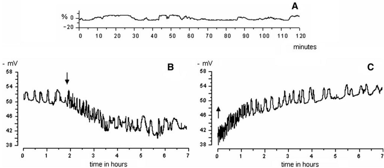
**FIG. 5.** Effect of experimenter on the BIOSCOPE signal. **A**, control signal in empty room (below 0.1 oscillations per minute); **B**, in presence of person in the room (about 0.2 oscillations per minute, 2–3 m from BIOSCOPE); **C**, after the person left the experimental room. Arrows show the moments the person came (**B**) and left (**C**) the laboratory.
