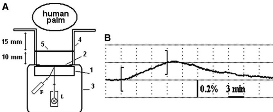
**FIG. 4.** Distant influence of the human palm on BIOSCOPE signals at the mechanical isolation of the sensor from an environment. **A**, scheme of experiment: labels 1–3, F, and L are the same as in Figure 1; 4, metallic tube closely fitting to the body; 5, thin metallic plate hermetically built in the tube. **B**, influence of the palm on the reflected light intensity. The brackets represent the time interval of the influence.
