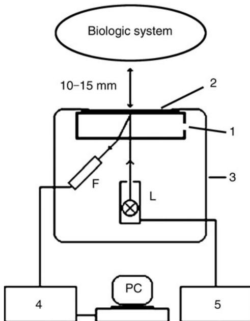
**FIG. 1.** Design of device complex BIOSCOPE. 1, glass plate of the thickness of 1–2 mm; 2, covering material (a dense black paper, thin opaque plastic); 3, metal case; L, light source (incandescent lamp or laser); F, photodetector (photo diode); 4, amplifier; 5, power unit; PC, personal computer: registration system.
